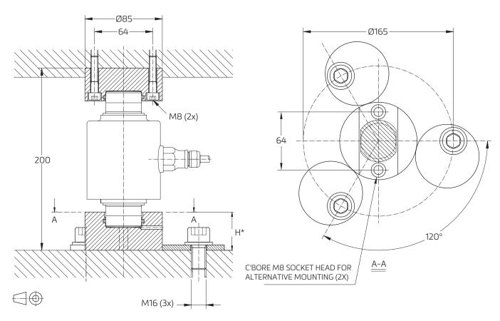
\*H = 52mm for RC3-30t, 42mm for RC3-40t and 42mm for both RC3D-30t and RC3D-40t
