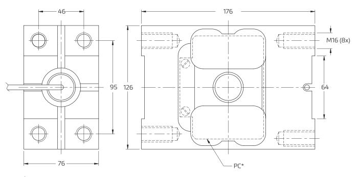
Mounting bolts M16 8.8; torque 200 Nm. Torque value assumes oiled threads. PC\* - Protective cover available on request. 6mm thick, two sides.
