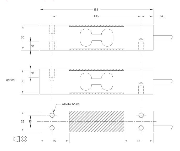
Mounting bolts M6 8.8; torque 10 Nm. Torque value assumes oiled threads.
