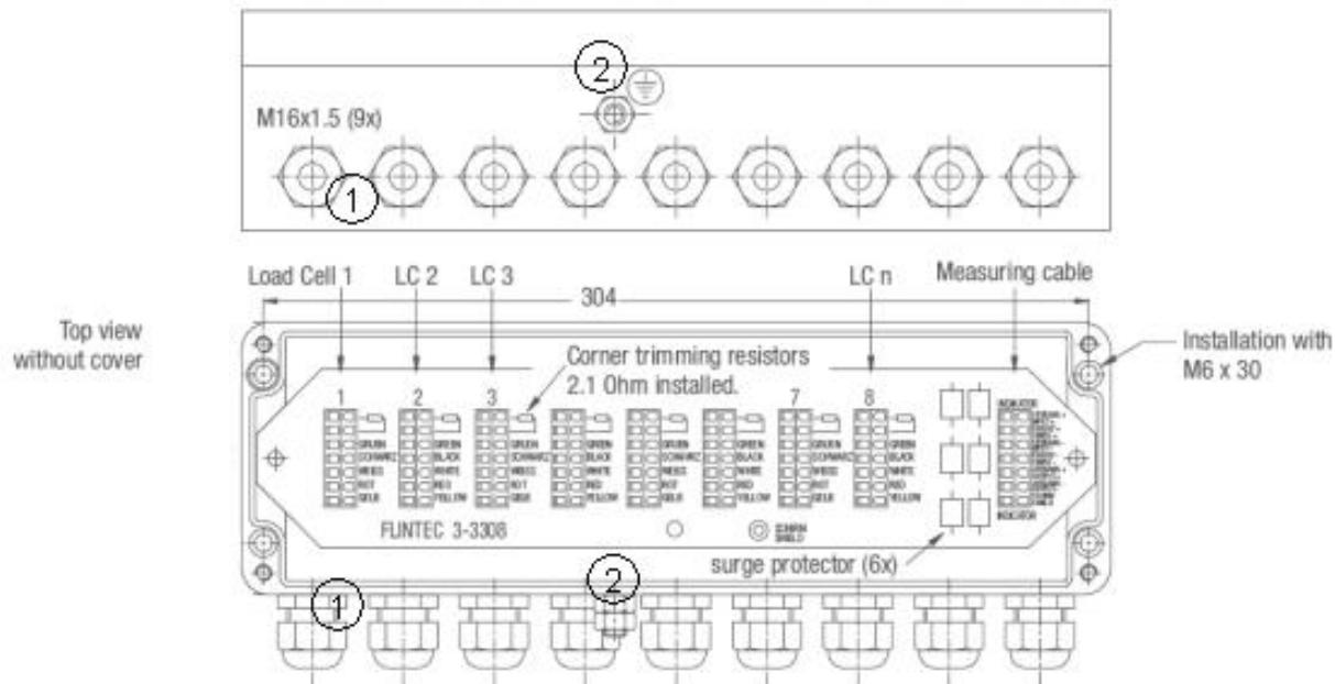
The earth screw (see (2) in fig.1) has to be connected to protective earth or you must establish an electrical connection to the weigh modules for potential equalisation. For doing this only the upper nut should be loosened and tightened again. The lower nut (= counter nut) and the earth screw with washer must not be rotated or loosened – the gasket is bonded! If loosened by accident the earth screw must be re-inserted and locked with some Loctite.
