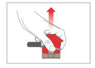
Pull upwards at the same time as pressing in the lever horizontally.
