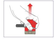
Pull upwards at the same time as pressing in the lever horizontally.
