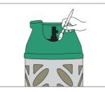
**5 Checking for leaks**
