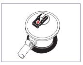
**2** Note that in the ON position, the flame symbol on the lever will be visible.
