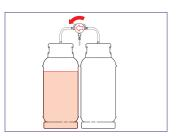
3 When the indicating arrow shows red, the control knob should be turned until the arrow points to the other cylinder. The empty cylinder should then be replaced.
