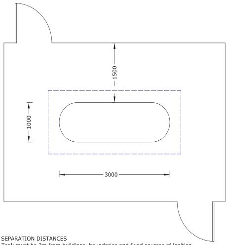
Tank base should extend at least 300mm around tanks i.e. 3600mm x 1600mm Minimum depth of 100mm concrete on a hardcore fill. For ease of maintenance it is recommended to concrete all area inside the compound
