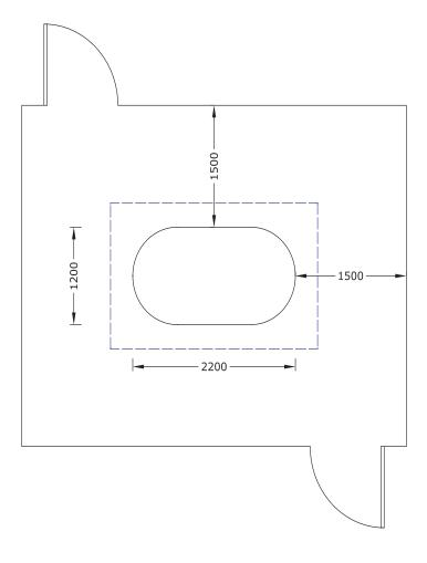
Tank base should extend at least 300mm around tanks i.e. 2800mm x 1800mm
