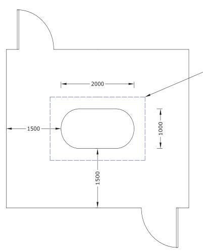
Tank base should extend at least 300mm around tanks i.e. 2600mm x 1600mm Minimum depth of 100mm concrete on a hardcore fill. For ease of maintenance it is recommended to concrete all area inside the compound
