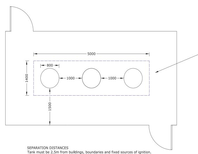
This may be reduced to 0.3m by using a firewall (normally on one side only).
