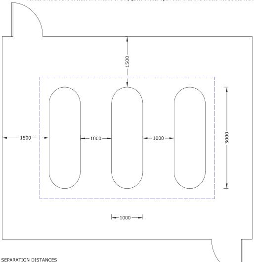
Tank base should extend at least 300mm around tanks i.e. 5600mm x 3600mm Minimum depth of 100mm concrete on a hardcore fill. For ease of maintenance it is recommended to concrete all area inside the compound
