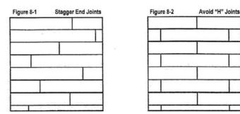
necessary), using appropriate fasteners. Denser species may require pre-drilling. Each succeeding row should be blind-nailed wherever possible.
