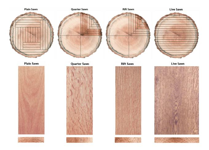
**Plain sawn** is the most common cut and was the standard for homes built the first half of the last century. Typically, two- to three-inch planks of red oak were used, featuring a "cathedral" pattern in the grain. Annual growth rings were very prominent, at a zero- to 35-degree angle.
