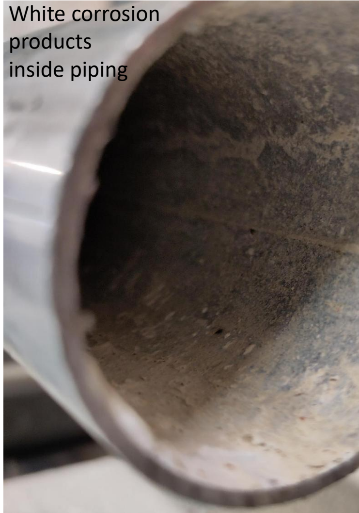
1.8 mm steel pipes protected from corrosion by a zinc coating. Installation 2014. Filled with tap water at 5 bar with pressure increase reported in 2015
