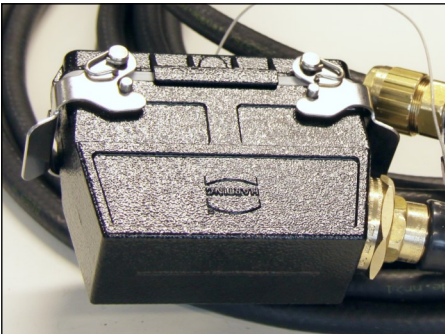
HAN plug connector with protective cover in use
