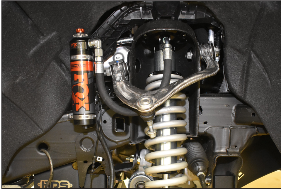
FIGURE 15A (WITH DSC RESERVOIR -PASSENGER SIDE)
