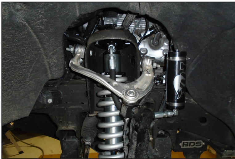
FIGURE 10 (NON DSC RESERVOIR - DRIVER SIDE)
