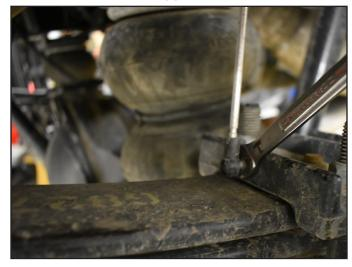
9. Install the provided spacers 136 into the ends of the air bag spacer and place the air bag spacer between the air bag and frame with the U cutout towards the center of the vehicle for the air ine. (Fig. 5 & 6). The spacers are not side specific. Fasten with OE hardware and Torque to 89 ft-lbs.
