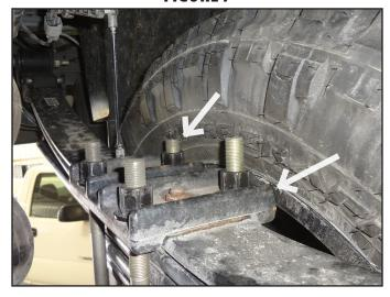
15. Recheck all hardware, check again at 500 miles, and again at regularly scheduled maintenance intervals. Check brake lines and ABS wires for proper clearance through steering sweep, use zip ties on the ABS wires if necessary. An alignment must now be performed.
