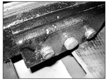
8. Install the new lift block. Install the new U-bolts and install the nuts, but do not tighten at this time.
