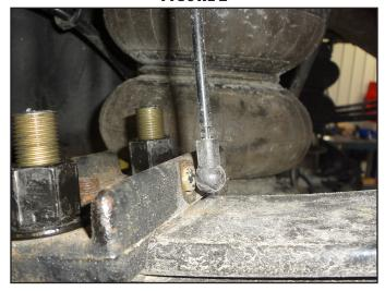
7. Lower the axle and removed the factory plastic center pin be carefull not to over extend the air bag air line. Replace with new metal pin. The pin will be a press fit. It may be necessary to take a rotary grinding tool to remove the sharp edge from the leaf pack to allow easier installation (Fig 3).
