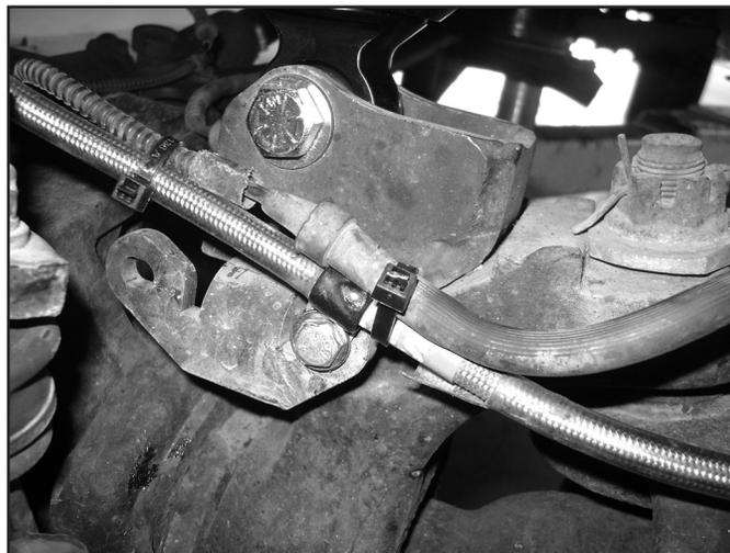
24. Install optional auxiliary shock in factory position with factory hardware if desired.
