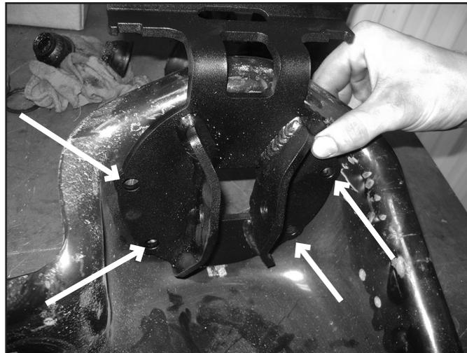
13. Mark the center of the holes, remove bracket, and drill out to 15/32" to 1/2". Make sure the drill does not damage the module on the driver's side (not present on all model year trucks).!
