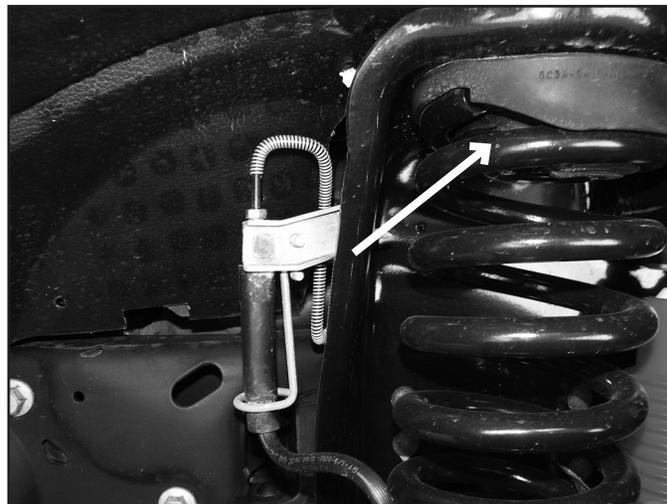
9. Remove the lower coil spring seat from the top of the axle, it will not be reinstated.
