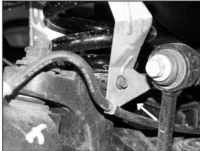
8. Lower the axle and remove the factory coil springs and upper coil spring isolator. Take care not to over extend any brake, ABS, or vacuum lines. (Fig 3)
