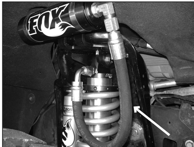
20. Remove the factory bump stop, remove the factory hardware that attaches the cup to the frame.
