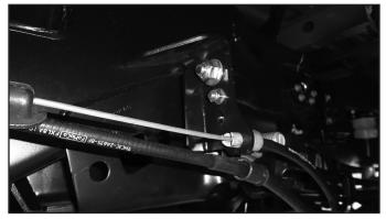
74. Install the passenger side E-brake cable into the bracket, make sure the tabs on the cable lock the cable into place.
