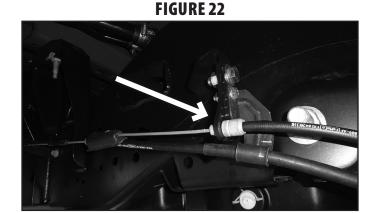
75. Remove the 3/8" bolt on the front leaf springs clamp. Install the E-brake clamp bracket with the new provided 3/8" bolt and nut from bolt pack 998 through the leaf spring clamp. Make sure the E-brake clamp bracket is towards the outside of the leaf spring. Tighten the 3/8" hardware with the spacer tube in between to 25 ft-lbs.
