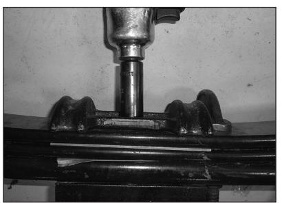
69. The OE upper U-bolt mount will be installed on the new leaf springs. Clamp the top and bottom of the new leaf springs near the center pin, but still allowing enough room to install the OE upper U-bolt mount. Remove the center pin from the new leaf springs and attach the OE upper U-bolt mount to the new leaf springs with the center pin. A pair of new center pins are provided incase the center pins in the new leaf springs strip out.
