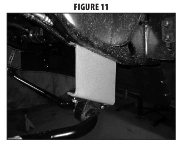
Install the sway bar link ends to the sway bar and secure with the OE hardware. Torque to 90 ft-lbs. 40.
