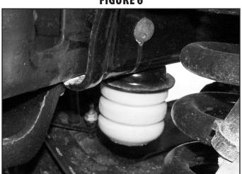
20. Position the cup on the provided bump stop extension, attach with 5/16" hardware from bolt pack #606. The alignment tab on the bump stop cup will fit in the second hole in the extension. Tighten to 30 ft-lbs.
