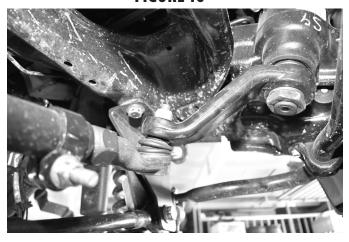
29. Install the new pitman arm, use the alignment mark made earlier. Thread locker factory nut and install with lock washer tighten nut to 332 ft-lbs. (Fig 17)
