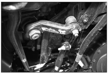
9. Disconnect the sway bar links from the sway bar. Retain all hardware. (Fig. 4)
