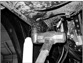
20. Grease new replacement bump stops and raise axle to press the bump stops into position. These will be a tight fit. It is easiest to lift the axle with a jack to compress the bump stops into position. (Fig. 9)
