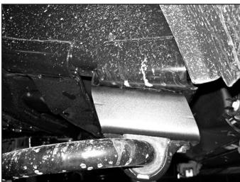
34. Reconnect the sway bar links with the factory hardware, torque to 60ft-lbs
