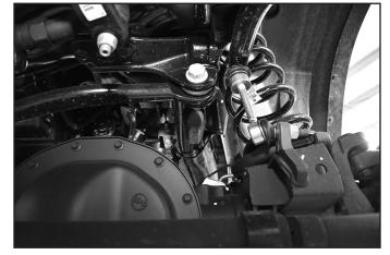
3. Raise the front of the vehicle and support the frame rails with jackstands. Do not support the vehicle by the radius arms, they will be removed during the installation.
