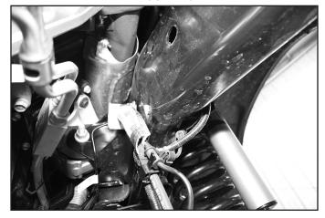
33. Install the sway bar drop brackets with factory hardware to the frame. The flat side of the bracket will face "out" and the brackets will offset the sway bar slightly forward. Attach the sway bar to the drop brackets with 3/8" hardware (Bolt Pack 422), tighten factory hardware to 43 ft-lbs and 3/8" hardware to 37 ft-lbs. (Fig. 20, 21)
