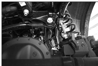
Raise the front of the vehicle and support the frame rails with jackstands. Do not support on the radius arms, they will be removed during the installation.
