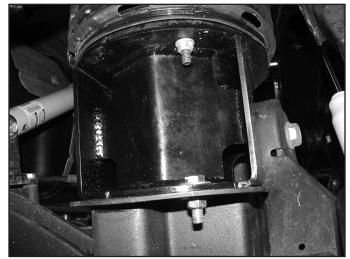
20. Install the shock eliminator bracket onto the shock using hardware in bolt pack 946 included in the shock box. Tighten 1/2" eliminator hardware to 75ft-lbs. Drill out the small hole inside the frame behind the shock mounting hole to 3/8". Install the shocks into the vehicle. Tighten 3/4" eliminator hardware to 120ft-lbs (Fig 12)
