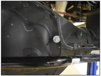
8. Remove E-brake bracket from the driver side frame in the wheel wheel for extra slack during installation, save hardware. (Fig 3)
