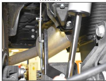
28. Attach the factory linkage stud to the linkage bracket with the provided nylock nut (BP359). Use the following image as a guide for your desired ride height. Pop the linkage rod back onto the stud. (Fig 19)
