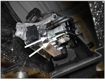
12. Disconnect the ride height linkage from the axle using a clip tool (Fig 5c).
