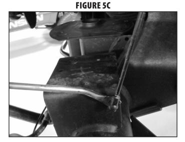
13. Disconnect the rear shocks and lower the axle, retain hardware. On the driver's side it is easiest to access the top hardware by cutting the inner fender well as shown. This trim procedure is not required but greatly aids in removal and installation of the shock (Fig 6, 7).
