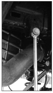
22. Remove the factory bump stops from the vehicle. (Fig 14)
