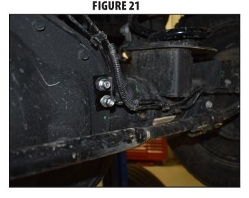
**31. 5" Lift Only, E-Brake Line Brackets:** Install the driver side rear brake line bracket to reattach the e-brake to the frame. (Fig 22)
