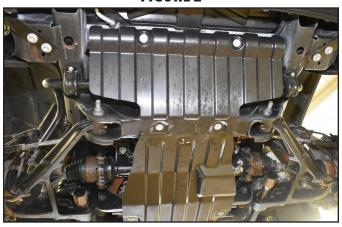
10. Disconnect the sway bar end links from the sway bar and then the lower control arms (Fig. 3). Discard the link assemblies.
