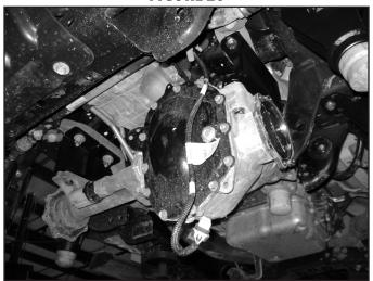
37. Locate the new rear cross member. Install the cross member in the rear lower control arm pockets with the factory control arm bolts/nuts. Run the bolts from rear to front. The center differential bracket will fit into the mount tabs on the cross member. Fasten the differential mount to the cross member with a 9/16" x 4" bolt, nut and 9/16" SAE washers (BP #586). Leave hardware loose (Fig. 27A).
