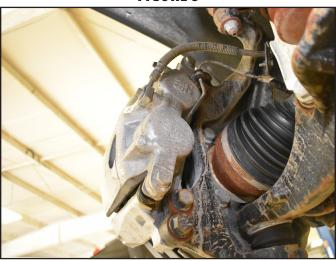
14. Carefully remove the hub dust cover. Save cover (Fig. 9).
