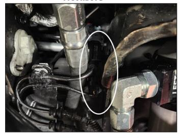
54. Once disconnected, you can install the reservoir using the two supplied billet clamps and screws. TO mount, utilize the slots in the bracket to locate clamps. Do not feed the clamps through the slots in the brackets. Torque the (4) four socket head cap screws to 19 IN-LBS. (Fig. 40)
