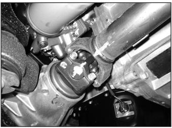
26. Remove the four bolts mounting the rear cross member to the rear lower control arm pockets (Fig. 18). Remove the cross member from the vehicle. The cross member and hardware will not be reused.
