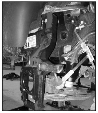
68. Locate the hub o-rings from the factory steering knuckle hub bores. Carefully remove the o-rings if still in the factory knuckle (Fig. 45) and install into the new steering knuckles.
