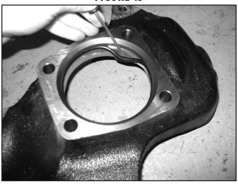
69. Locate the factory driver's and passenger's brake dust shields. They need to be modified to provided adequate brake caliper clearance. Make a cut line by following the straight edge on the caliper side of the shield all the way to the bottom edge of the shield (Fig. 46). Cut the shield along the line.
