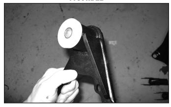
33. Locate the 4 housing bolts to be removed. Remove the four bolts, place the bracket in position and fasten with new 10mm x 40mm bolt and washers (BP #586). The bracket gusset will be toward the bottom of the differential (Fig. 23). Use thread locket on the bolt threads and torque to 59 ft-lbs.
