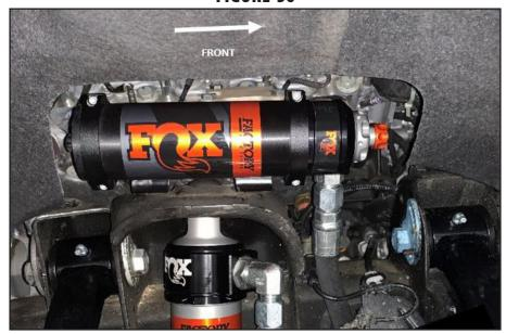
51. Using the supplied hardware, attach shock to upper mounting, using a washer on both the bolt and the nut. Ensure that the reservoir bracket is between the top of the shock bucket and the supplied hardware. (Fig. 37). Torque to 48 ft-lbs.
