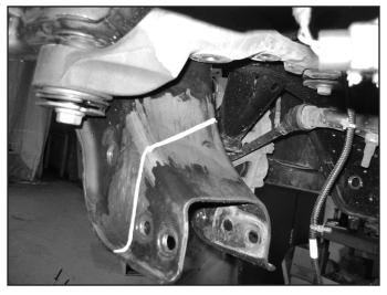
31. Using a reciprocating saw (recommended), cut-off wheel, or plasma cutter, cut the pocket along cut lines. Remove any burrs or rough edges and paint any bare metal to prevent corrosion.
