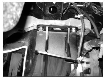
36. Using an appropriate jack, raise the differential up into the vehicle. Align the differential mounting holes to the new driver's and passenger's side differential brackets. Fasten to the driver's side mount with 1/2" x 3-1/2" bolts, nuts and 1/2" SAE flat washers (BP #586). Fasten the passenger's side 1/2" x 1-1/2" bolts, nuts and heavy 1/2" (large OD) washers. Snug up hardware, but do not tighten (Fig. 26).
