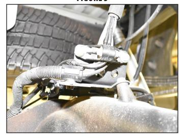
13. The passenger's side bump stop bracket on the axle must be trimmed slightly to add clearance for the new larger rear shocks. Grind the inside front corner to gain approximately 1/4" of clearance (Fig. 6). Paint bare metal to prevent rust.
