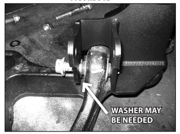
45. With both new torsion bar bracket installed on the factory control arms, install the control arms in the cross members. Fasten the control arms with the provided 18mm x 120mm (front) and 18mm x 140mm (rear) bolts, nuts and 3/4" SAE flat washers (BP #585). Run the front bolts front-to-rear and the rear bolts rear-to-front (Fig. 32). Leave hardware loose. These bolts will be torque with the weight of the vehicle on the suspension.
