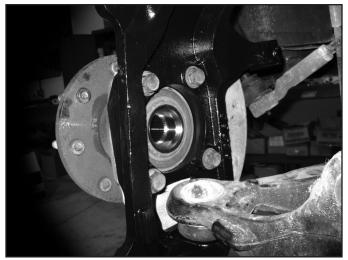
72. Run the ABS line around the back side of the tie rod of the steering knuckle and up to the wire connector on the frame. Reconnect the wire and reattach it to the original place on the frame. Attach the ABS line to the back side of the knuckle near the tie rod end using a wire clamp and a 1/4" x 5/8" bolt, flat washer and lock washer (BP# 877) (Fig. 49). Torque 1/4" hardware to 86 in-lbs.
