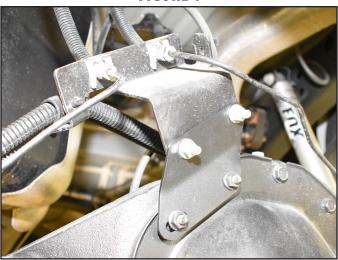
12. Install the rear ABS line relocation bracket to the differential using the factory hardware. Using the provided 1/4" hardware (BP #873) attach the rear brake line bracket to the relocation bracket (Fig. 5). Additional wire clips may need to be undone to add enough slack for the ABS lines, use the zip ties where needed.
