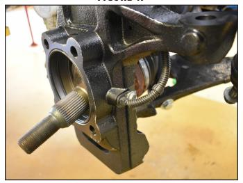
71. Install the hub assembly, O-rings, and dust shield into the appropriate steering knuckle (Fig. 48). Fasten the hub to the knuckle with the factory bolts. Apply thread locker to the threads and torque the bolts to 133 ft-lbs.
