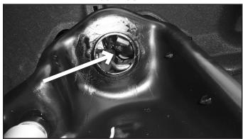
13. Place the upper coilover mounting bracket up to the upper mount. Rotate the bracket so that the reservoir bracket is parallel with the frame. (Fig 6)
