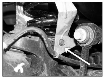
8. Lower the axle and remove the factory coil springs and upper coil spring isolator. Take care not to over extend any brake, ABS, or vacuum lines. (Fig 3)
