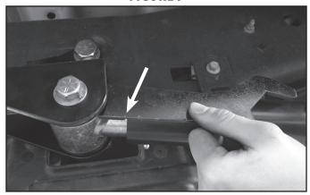
26. After the desired force is set, lock off the jam nut with the two provided Jam Nut Wrenches and repeat this process on the other Recoil Traction Bar. Note: Never unthread the forged flex end past 1-1/2" of adjustment. This can cause thread damage and weaken the joint. See Figure 10.
