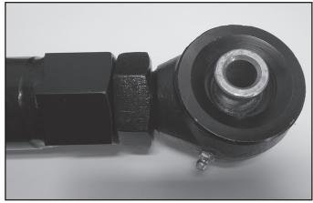
8. Attach the Traction Bar to the axle bracket with a 9/16" x 4" bolt, 9/16" nut and 9/16" SAE washers from Bolt Pack 964. Install the traction bar so that the Forged Flex End (A171) is mounted to the axle bracket. Leave mounting hardware loose at this time
