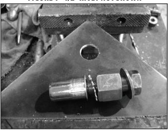
FIGURE 1 - 1/2" RIVET NUT SHOWN
