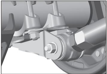
9. Measure the length of the bar from the center of the bolt at the axle to the center of the sleeve at the traction bar end (02869). The length should be approximately 59-3/4". If not, press firmly on the traction bar end to seat the springs.
