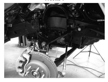
11. Install new control arm with factory cam bolts. Snug, but do not torque bolts. Do not install the upper ball joint cap at this time. Do not attach to the steering knuckle at this time. (Fig 5)
