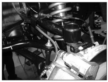
16. Attach modified factory brake line bracket to the upper control arm with ¼" hardware. Tighten to 12 ft-lbs. Cycle the steering to ensure that the brake line clears the sway bar components. Rotate bracket if necessary. (Fig 8a, 8b)
