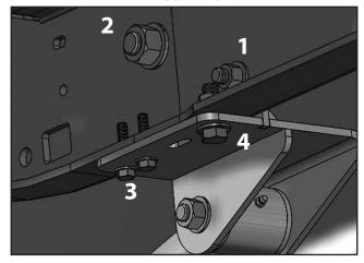
25. Attach the traction bar slider end (02869) to the frame bracket using a 9/16" x 4" bolt, 9/16" nut and 9/16" SAE washers from Bolt Pack 964. Note: The traction bar slider end will slide out of the Recoil Traction Bar to attach to the frame mount. If it cannot slide out far enough, spin the bar so that it un-threads from the Forged Flex End.
