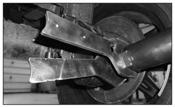
43. Use the levels on the wrench to gauge how much force is inputted into the Recoil Traction Bar. The wrench is designed to be used at the traction bar slider end as shown in Figure 23. Make sure the wrench is pressed firmly against the bushing / tube for an accurate measurement.
