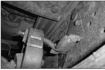
30. 1999-2010 Models Only (Exhaust Hanger Modification): Rotate the exhaust hanger down and remove the hanger from the rubber isolator. Using a vice and a hammer, bend the hanger so that it becomes flatter, pointing more towards the ground when installed up side down. The hanger and mounting plate should form approximately a 110 degree angle. Note: Do not bend the hanger too far such that it will not support the exhaust.
