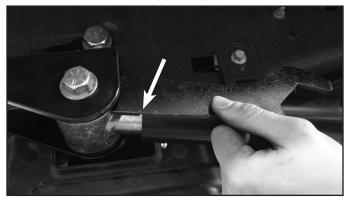
46. Utilize the Jam Nut Wrench to set a desired force setting (Minimum of the First Level). Depending upon suspension setups, different spring preload may need to be tried to find a good setup to reduce axle wrap. After the desired force is set, lock off the jam nut with the two provided Jam Nut Wrenches and repeat this process on the other Recoil Traction Bar. Note: Never unthread the forged flex end past 1-1/2" of adjustment. This can cause thread damage and weaken the joint. See Figure 27.
