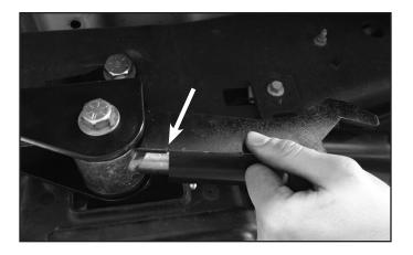
34. After the desired force is set, lock off the jam nut with the two provided Jam Nut Wrenches and repeat this process on the other Recoil Traction Bar. Note: Never unthread the forged flex end past 1-1/2" of adjustment. This can cause thread damage and weaken the joint. See Figure 10.
