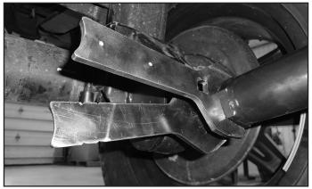
31. Use the levels on the wrench to gauge how much force is inputted into the Recoil Traction Bar. The wrench is designed to be used at the traction bar slider end as shown in Figure 6. Make sure the wrench is pressed firmly against the bushing / tube for an accurate measurement.
