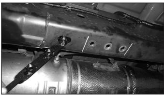
18. Attach the frame bracket to the frame rail with three of the 1/2" x 1-1/2" bolts and 1/2" SAE washers from Bolt Pack 963. Torque the 1/2" bolts to 60 ft-lbs.
