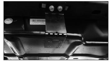
11. Remove the two bolts that are attached to the upper part of the fuel tank skid plate support that was just cut. Remove the two J-nuts from the frame rail.
