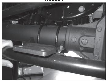
4. Install outer brackets as shown. Note: The flashing on the tie rod end forgings may cause interference with the brackets. Give them a slight tap, or rotate them on to fit over the tie rod end. Adjust hole center to center bracket hole centers to 20-1/8" stabilizers. Install 5/16" u-bolts, washes, and nuts, tighten to 18 ft-lbs. (Fig 2)
