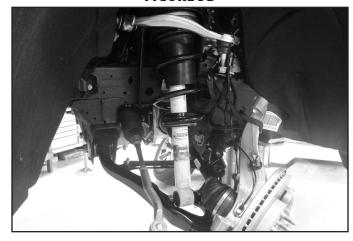
9. Remove the two lower strut bar pin bolts (Fig. 6). Lower the control arm with the jack so there is enough room to remove the factory strut.
