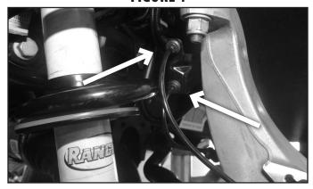
8. Support the lower control arm with a hydraulic jack and remove the nut from the upper ball joint (Fig. 5A). Dislodge the rod end taper from the knuckle. Allow the knuckle to swing rearward out of the way (Fig. 5B). **Denali Models Only:** Remove the sensor ball stud from the control arm.
