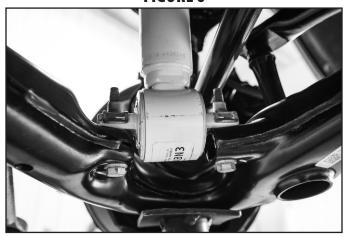
10. Remove the three nuts attaching the strut to the frame (Fig. 7). Remove the strut from the vehicle. DO NOT remove the center strut rod nut. Discard the nuts, they will not be reused.
