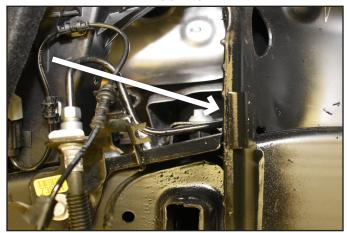
13. Install the new upper control arm to the vehicle using the **new provided 14mm bolts, washers, and nuts and using thread locker.** Run the bolt with a washer from the inside out of the strut bucket outwards with a washer and nut on the outer bushing washer surface. Do this for the front and rear control arm mounts. (Fig. 10) Snug up hardware.
