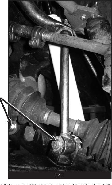
3. With the links completely installed, tighten the 3/8 hardware to 30 ft-lbs and the 5/8" hardware to 75 ft-lbs.
