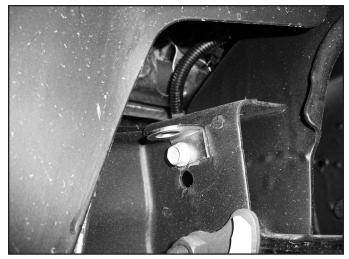
8. Run the end of the new brake line through the new bracket at the frame and attach it to the OE hard line. Tighten the fitting securely. Retain the brake line to the bracket with the new retaining clip (5188). Adjust the bracket so the brake line does not rub against the upper control arm cam bolt and torque bracket bolt to 20 ft-lbs (Fig 4).
