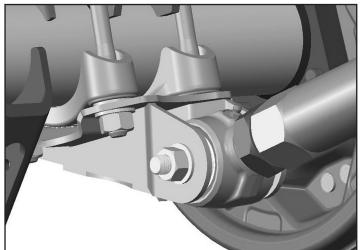
Measure the length of the bar from the center of the bolt at the axle to the center of the sleeve at the traction bar end (02869). The length
