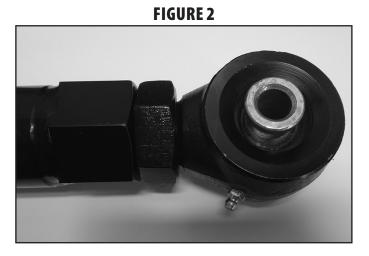
8. Attach the Traction Bar to the axle bracket with a 9/16" x 4" bolt, 9/16" nut and 9/16" SAE washers from Bolt Pack 964. Install the traction bar so that the Forged Flex End (A171) is mounted to the axle bracket. Leave mounting hardware loose at this time
