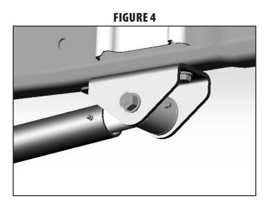
18. Grease all bushings and the Recoil Traction Bar before use. Do not over grease the Recoil Traction Bar, it is recommended to grease the Recoil Traction Bar one pump of grease every 10,000 miles.
