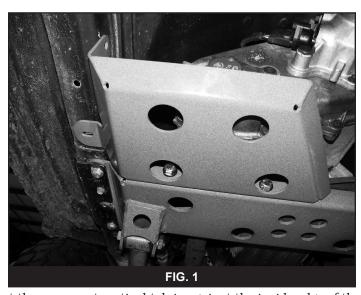
Adjust the skid plate so that the rear-most vertical tab is against the inside edge of the uni-body frame rail (Fig 2) and the bottom of the skid plate is flush with the bottom of the crossmember. Torque the  $\frac{1}{2}$ " bolts to 65 ft-lbs. Note: In some cases there may be lines, hoses or wires that need to be adjusted out of the way for clearance of the rear-most mounting tab against the frame.
