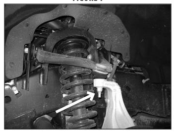
6. Remove the two bolts attaching the upper control arm to the vehicle. (Fig. 2)
