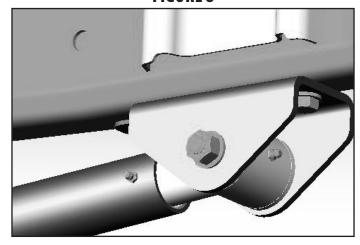
19. Grease all bushings and the Recoil Traction Bar before use. Do not over grease the Recoil Traction Bar, it is recommended to grease the Recoil Traction Bar one pump of grease every 10,000 miles.
