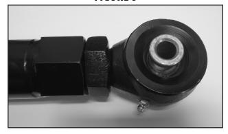
10. Attach the Recoil Traction Bar to the axle bracket with a 9/16"x 4" bolt, 9/16" nut and 9/16" SAE washers from Bolt Pack 964. Install the Recoil Traction Bar so that the Forged Flex End (A171) is mounted to the axle bracket. Leave mounting hardware loose at this time.
