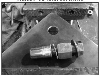
FIGURE 1 - 1/2" RIVET NUT SHOWN
