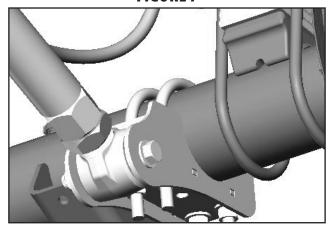
11. Measure the length of the bar from the center of the bolt at the axle to the center of the eye on the Forged Flex End (A171). The length should be approximately 59-3/4" +/-0.25". If not, press firmly on the traction bar slider end to seat the springs.
