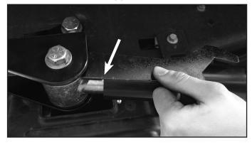
27. Utilize the Jam Nut Wrench to set a desired force setting (Minimum of the First Level). Depending upon suspension setups, different spring preload may need to be tried to find a good setup to reduce axle wrap. After the desired force is set, lock off the jam nut with the two provided Jam Nut Wrenches and repeat this process on the other Recoil Traction Bar.
