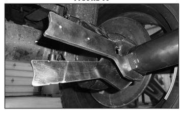
24. Use the levels on the wrench to gauge how much force is inputted into the Recoil Traction Bar. The wrench is designed to be used at the traction bar slider end as shown in Figure 11. Make sure the wrench is pressed firmly against the bushing / tube for an accurate measurement.
