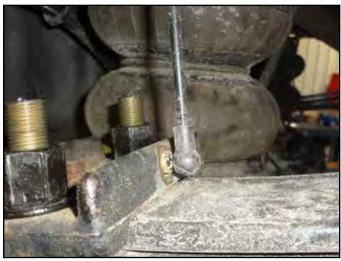
**10. 4" Kits ONLY:** Lower the axle and removed the factory plastic center pin. Replace with new metal pin. The pin will be a press fit. It may be necessary to take a rotary grinding tool to remove the sharp edge from the leaf pack to allow easier installation (Fig 6).
