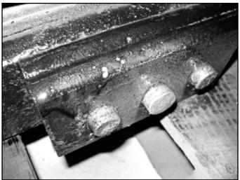
11. Lower the axle and install new lift block, with the small end of the block towards the front of the vehicle (Fig. 7). Install new U-bolts and install the nuts, but do not tighten at this time.
