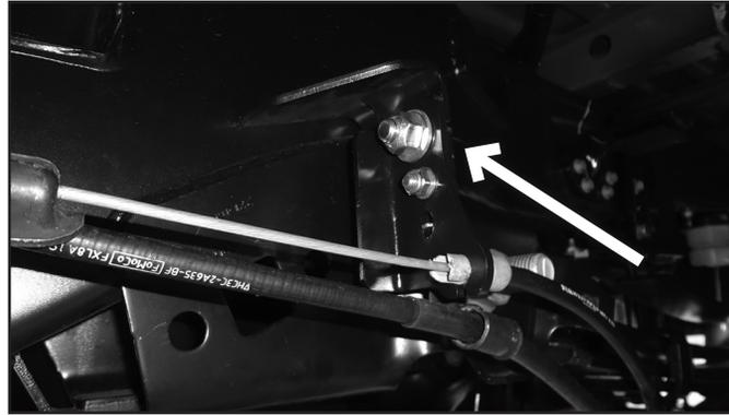
62. Install the passenger side E-brake cable into the bracket, make sure the tabs on the cable lock the cable into place (Figure 21).
