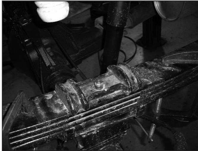
50. Remove the factory lift block. It will not be reused.
