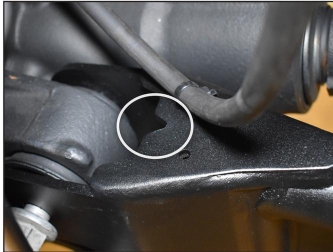
15. Working on one side of the vehicle at a time, remove the stock radius arm and replace with the new one. Install cams into the lower slots with new 18m hardware, and use new 18mm nut on the driver's side upper mount at the axle. The cam will be offset towards the rear of the vehicle as shown in the bottom image of Figure 9B.
