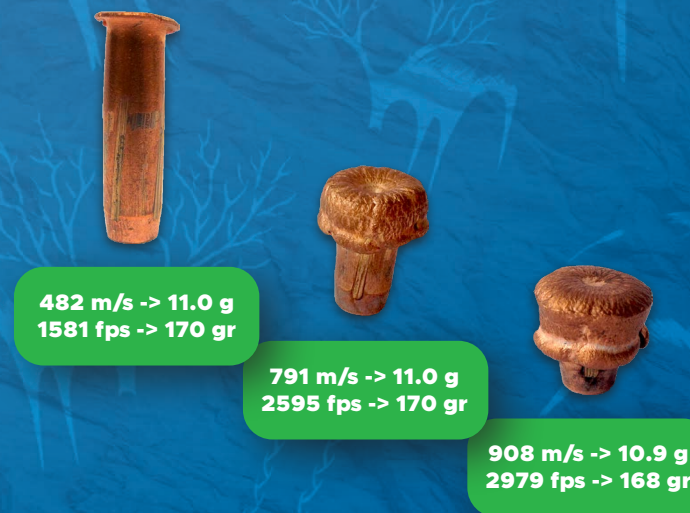
Mushrooming of .30 Naturalis –bullet with different point of impact velocities
