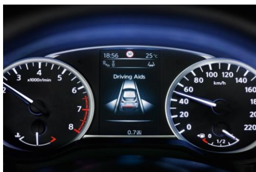
5" TFT display combimeter
