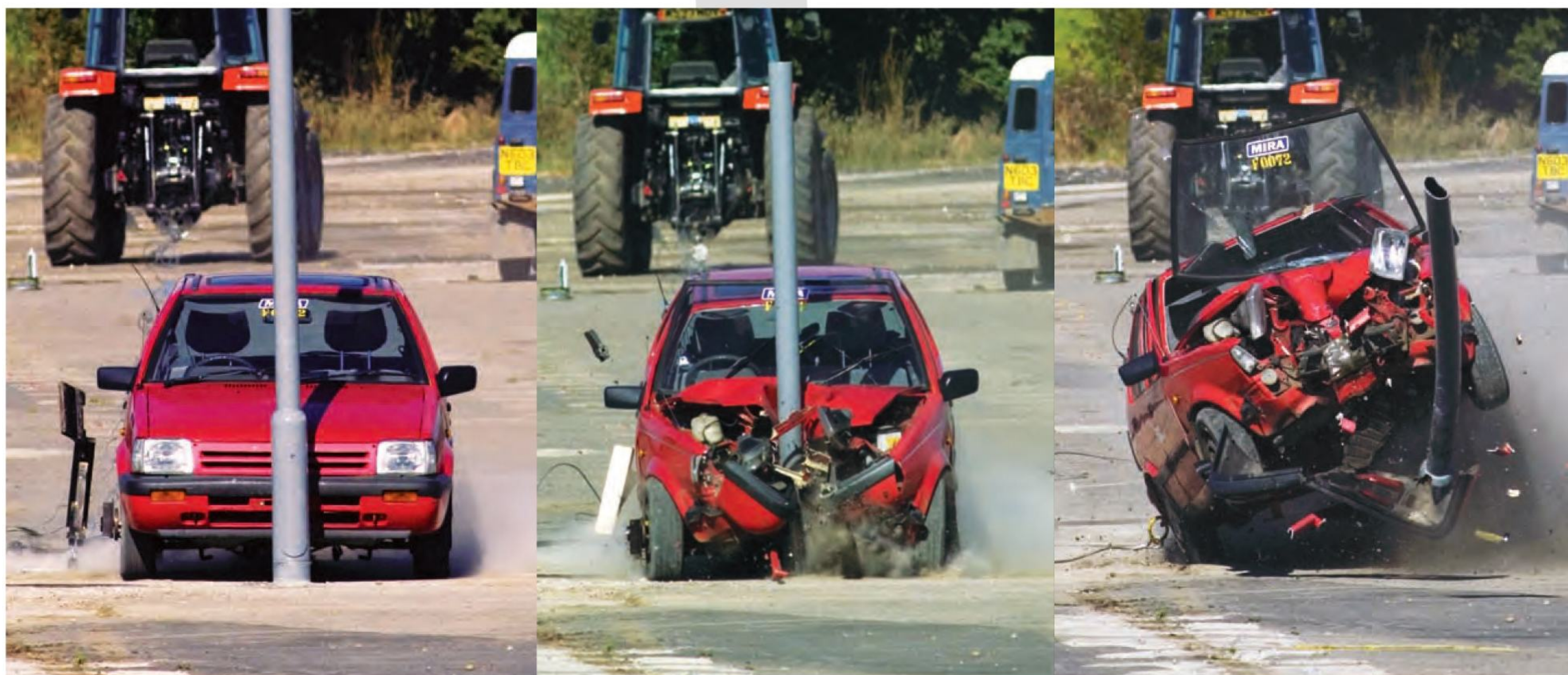
Car impacting a steel post at 100kph
