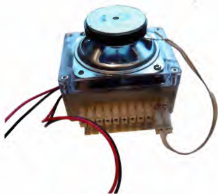
11. Sound module with top-mounted speaker using enclosure as sounding board. Pins 1 & 2 on the right of the 12-way connector are reserves for the loudspeaker outputs.'
