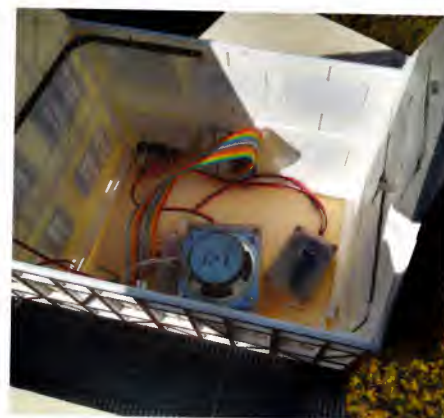
13. Half-built replacement Vollmer station showing the switch cluster, PSU and sound box, waterproof speaker and strip LED lighting.
