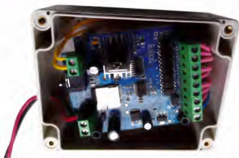
12. Sound board floating in enclosure supported by the trigger wires.
