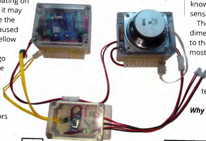
14. Sound Modular System: PSU (centre) to Sound Box only (left) and Sound Box plus Speaker (right)
