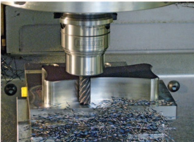
Standard / Standard APC 20-A Ø 3 - 20 mm
