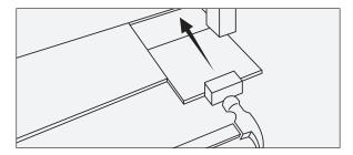
Internal expansion gaps are required at doorways/thresholds and rooms exceeding 20m x 15m.
