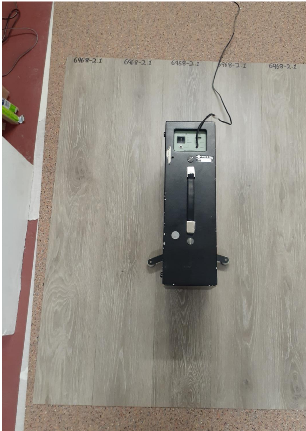
Figure 3 - LVP/T 2.5 mm CN plank construction with 2 mm Damtec colour underlay on base floor
