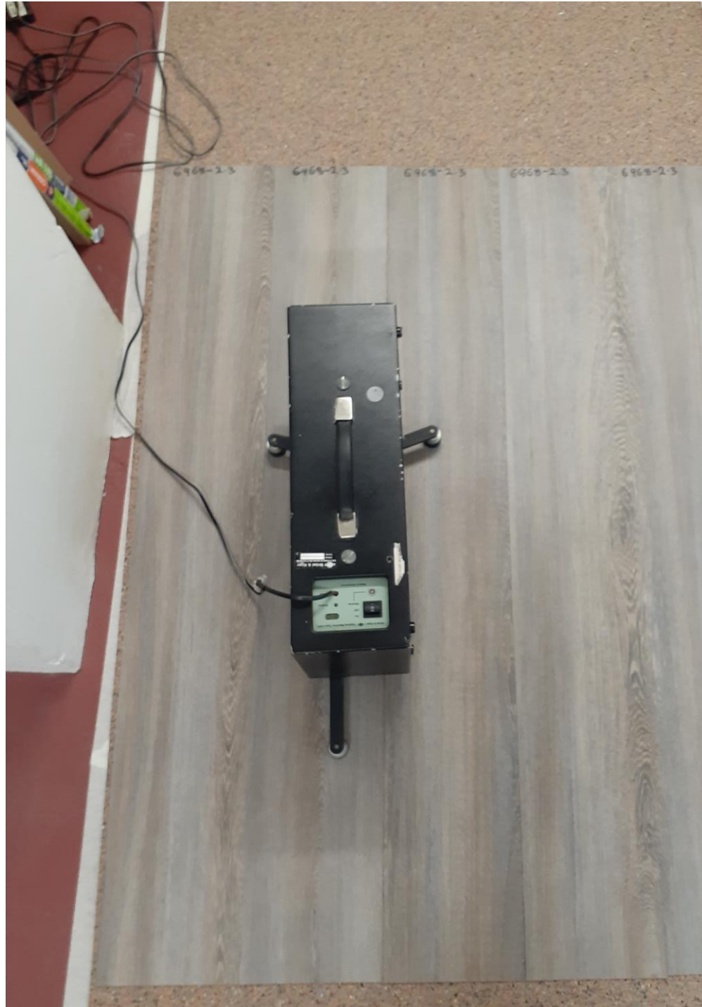
Figure 3 - LVP/T 2.5 mm EU plank construction with 2 mm Damtec colour underlay on base floor
