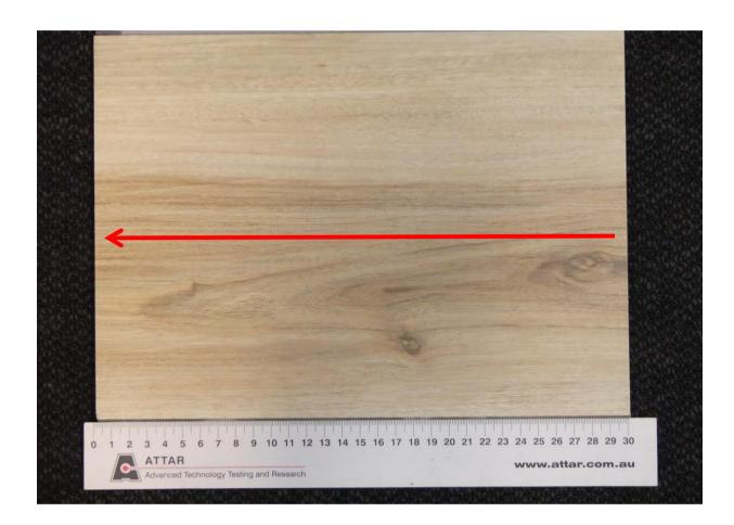
Figure 1: GH Hybrid 6.5mm / 0.5mm Wear Layer plank Arrow indicates direction of testing
