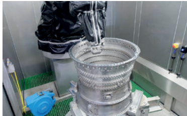
Waterjet stripping (coating removal)
