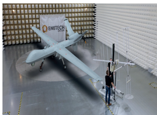
Full-scale UAV EMC testing — large anechoic chamber
