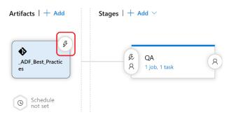
Enable the "Continuous deployment trigger. In the example below, we selected adf\_publish as filter branch. This mean, a deployment will be triggered whenever there is commit on the adf\_publish branch.
