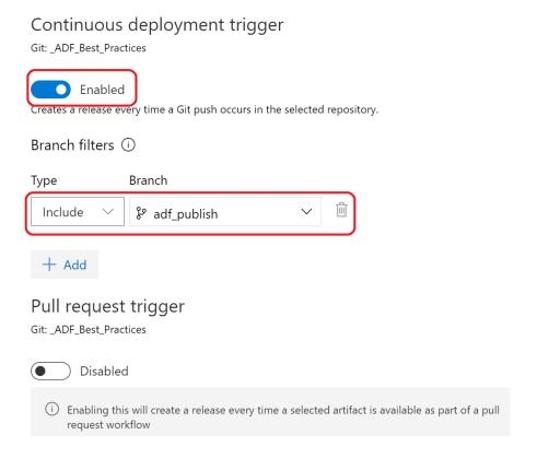
At this point, you can make some changes to you Data factory in the DEV branch and create a pull request. Once the reviewer approves the pull request and completes the merge in the collaboration branch, you can publish the change to the Dev environment in Azure Data Factory. This will automatically trigger a deployment to your QA environment.
