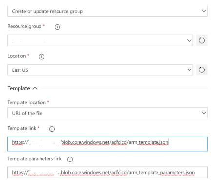
The override template parameter section allows to define the parameters in the target environment. We recommend having one parameter template file per environment.
