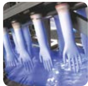
► Dipping in progress
